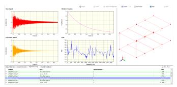
Signal Processing tab during impact hammer test.
