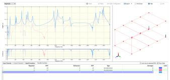
Transfer Functions tab during impact hammer test.
