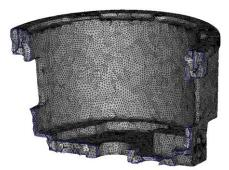
Fig. 4 Resulting 10-noded tetrahedron mesh
