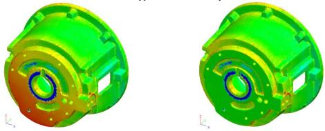
Fig. 8 The differences before (left) and after (right) the first mesh deformation
