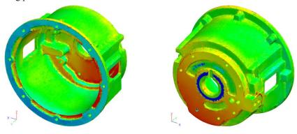
Fig. 6 The difference between the measured and CAD geometry.
