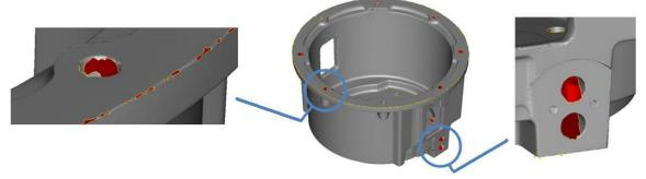
Fig. 3 Detail views of typical scan surface mesh imperfections: non-watertight edges (left) and incomplete hole or slot information (left and right).
