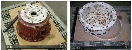
Fig. 2 Images showing the lantern housing during the digitizing process.
