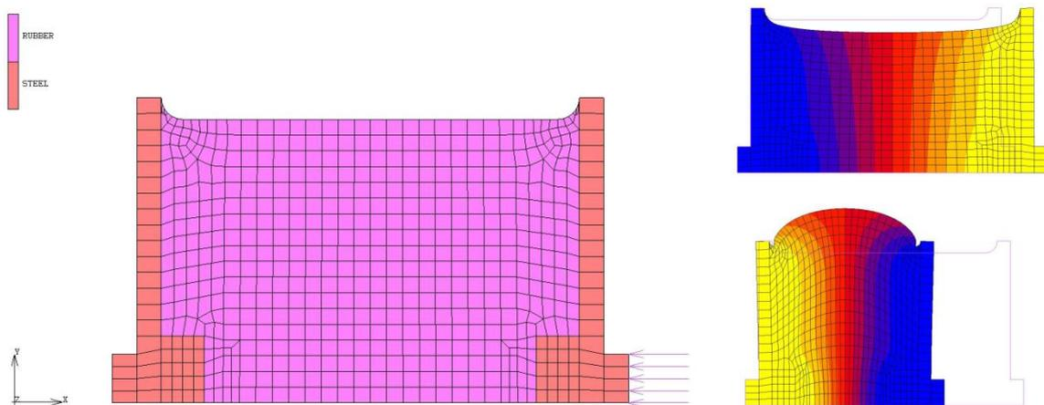
The parameter identification process converged to stable values for the Ogden parameters in five iteration steps. The overall improvement in correlation between the simulated and measured reaction force curves, due to the optimization of the Ogden material parameters, is presented below. The satisfactory correlation for the reaction force curve of the optimized FE-model shows that the Ogden parameters were correctly identified.
